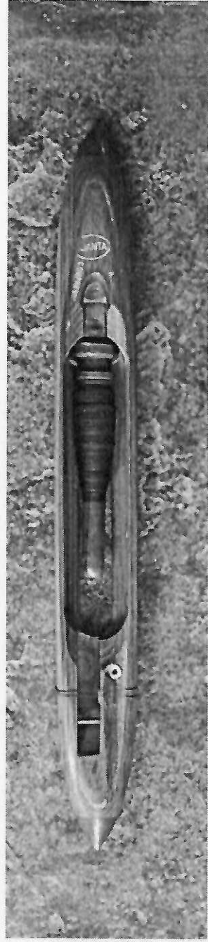
Flying shuttle loaded with pirns.
