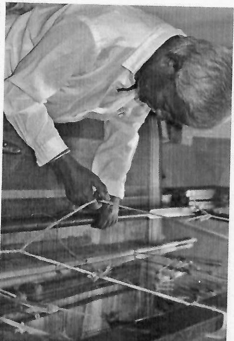
After the thread is positioned, the flying shuttle is again pushed through the yarn.
