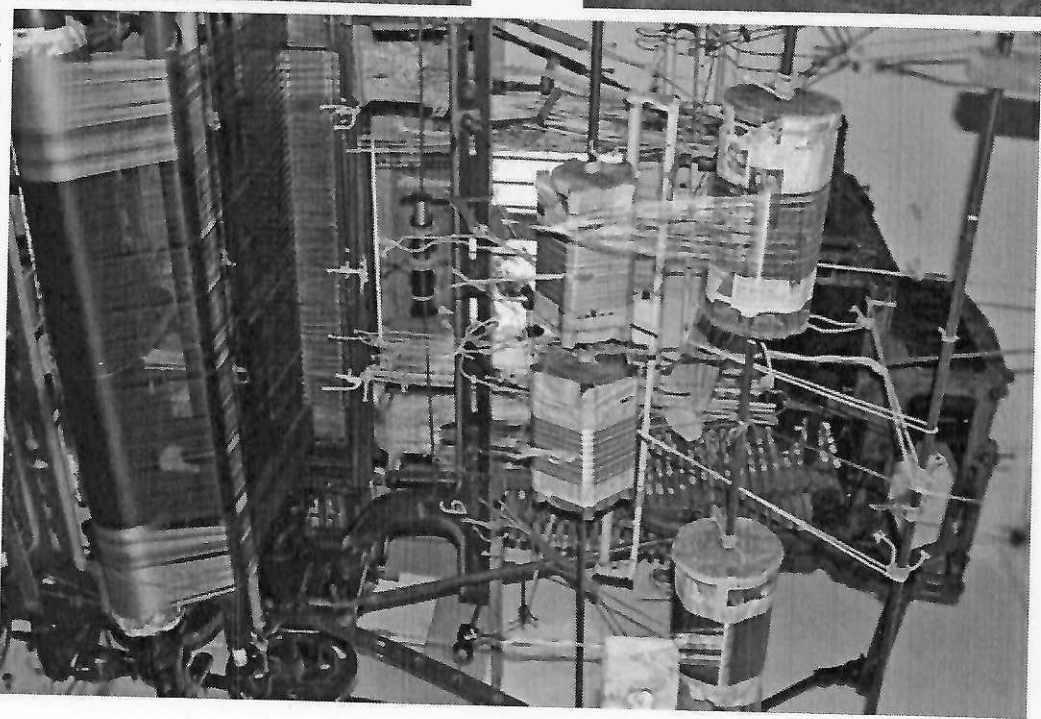
Dobby Loom allows the manufacture of complex patterns.
