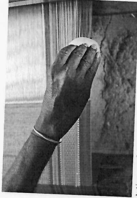
After the thread is positioned, the flying shuttle is again pushed through the yarn.
