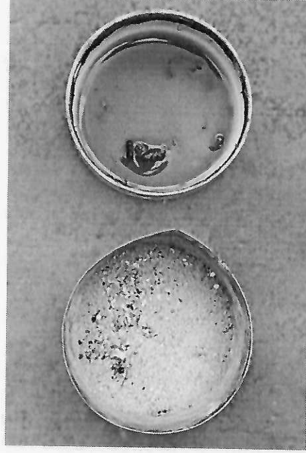
Wood ash and natural gum used during joining of two different threads together.
