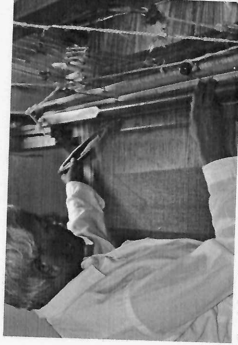
Loaded pirn is inserted into the flying shuttle.
