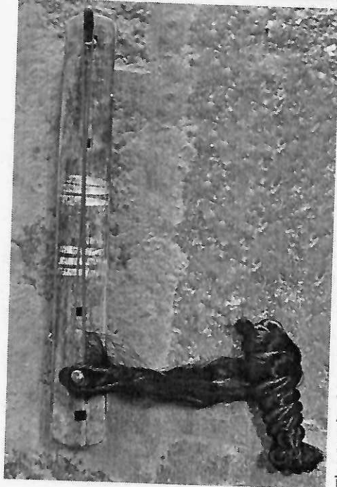
Empty Pirns winded manually with silk thread.
