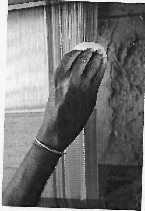
Artisan applying wax to the unweave yarn for smoothing the weaving process.
