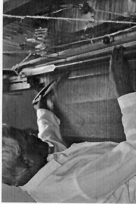
The flying shuttle is then passed through the divided part of the yarns to interweave and create a pattern.
