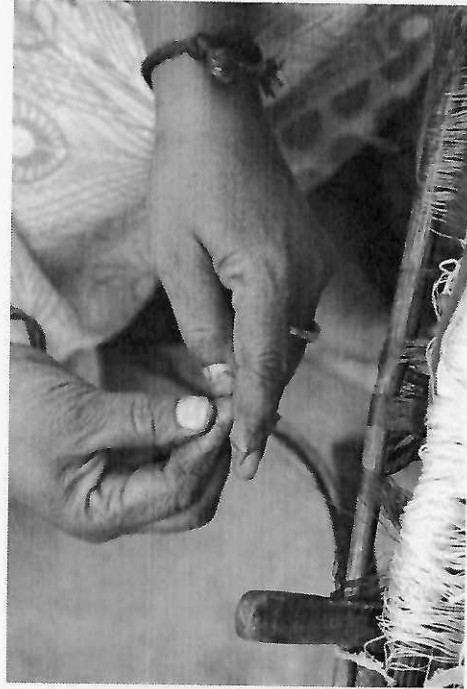
With the help of wood ash and natural gum the threads are linked with one another.
